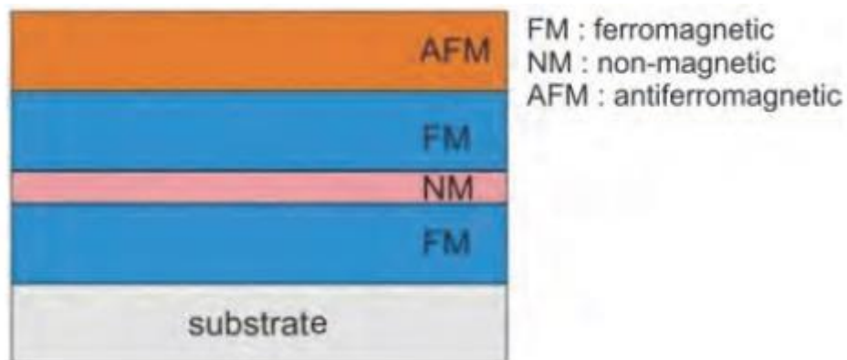
Figure 16 - Schematic representation of a GMR spin-valve sensor. Adapted from Ramli et al 89 .
